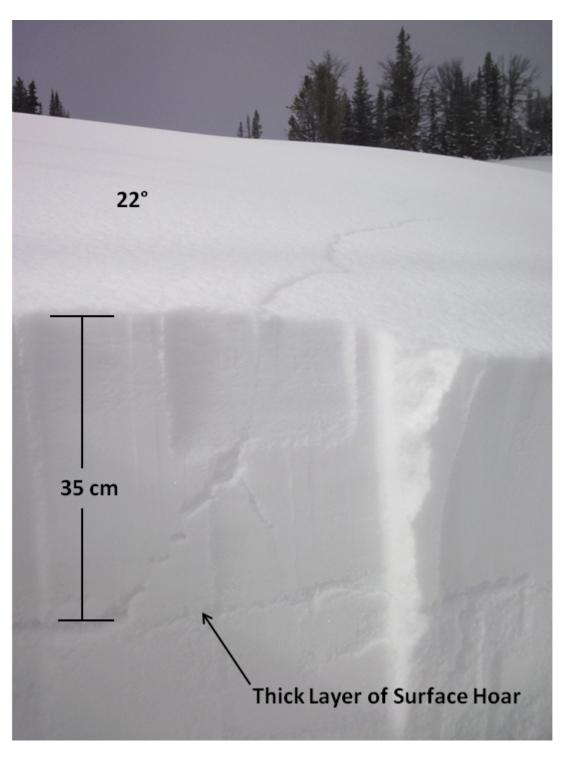
As we skinned up the slope we got a large "whumph" and crack that propagated about 75 feet uphill. We dug into the crack and saw it was collapsing on a 1.5cm thick layer of well developed, feathery, surface hoar. This is Bulls-eye information that the snowpack is unstable. We made a video of the snowpit too: http://www.youtube.com/watch?v=NDthVJsSFjE Photo: GNFAC
