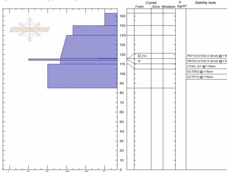
Notes: Prior pit to this lower on slope, at top of steeper meadow had ECTNs at storm interfaces, no propagation, or obvious SH layers. \ obvious until CT, and then ECTP 13 was a bit of a surprise. Shorter PST cut (15/100) was result of placing slab from previous test PST, essentially doubling the load.
