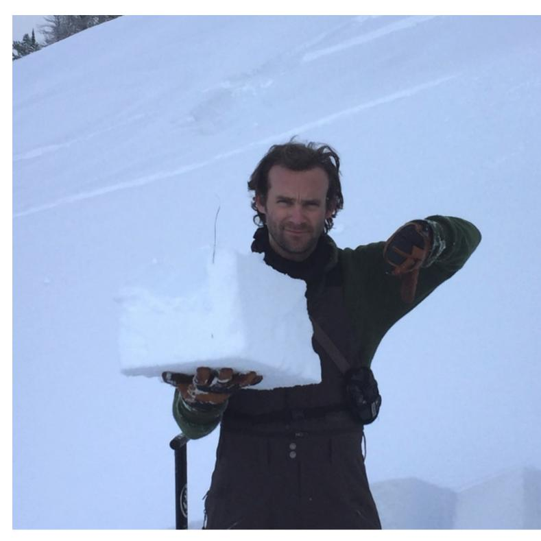
Stability test results were poor in Taylor Fork on Friday. There is 2-1/2 feet of snow on the ground, and it's breaking in two spots: a foot under the surface on surface hoar, and sugary facets near the ground. Both broke at the same time; ECTP13. It will not take much snowfall to tip the scales towards avalanches. Photo: B. Nobel
