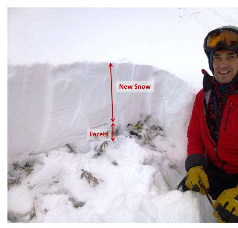
This was taken this morning (Wed) at Bridger Bowl after we issued an Avalanche Warning. Over 3 inches of SWE got piled onto a base layer of facets. This layer is breaking very, very easily. I was able to get entire slopes to fracture and whumph with simple ski turns. Photo: GNFAC
