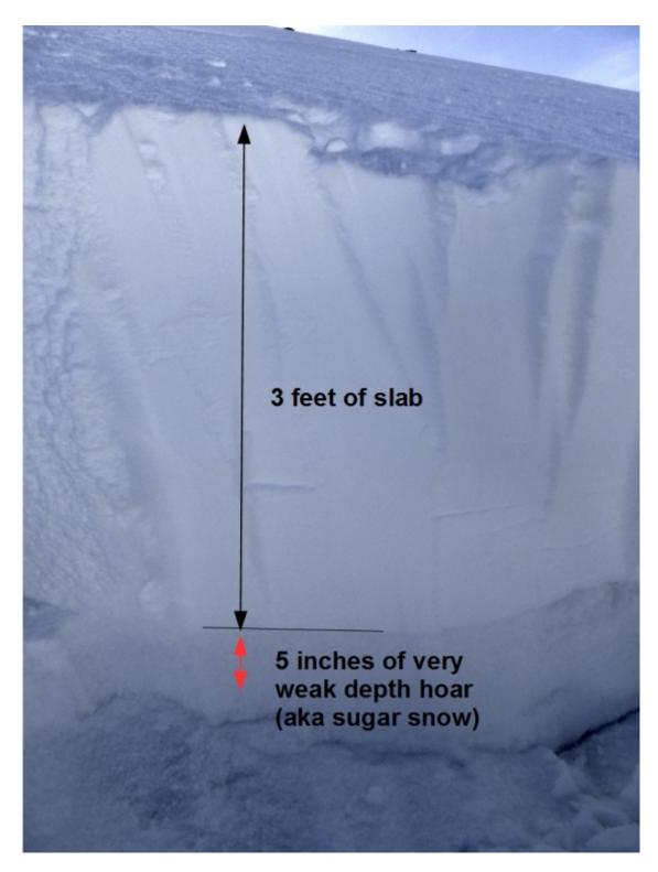
This slope had very thin snow considering the nearby Fisher Creek SNOTEL has over 10 feet of settled snow. This thin snowpack led to the formation of very weak **depth hoar** (6-10mm in size and Fist+ hardness). Photo: GNFAC
