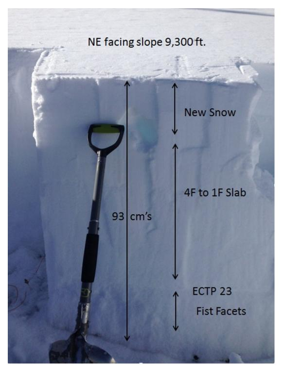
This snowpit was dug on Yellow Mountain north of Big Sky. The snowpack structure in this area is poor, with facets near the gound being the layer of concern. It's becoming harder to impact this layer, but it's still capable of propagating a fracture and producing avalanches. Photo GNFAC
