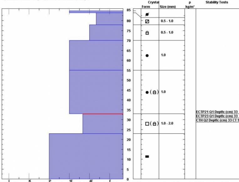
I K P 1F 4F F U Notes: This snowpit has similar structure to the Football Field on Saddle Peak. The ECTP made sense given the two natural slides earlier on thinner sp cornice drops as triggers. Danger felt MODERATE.
