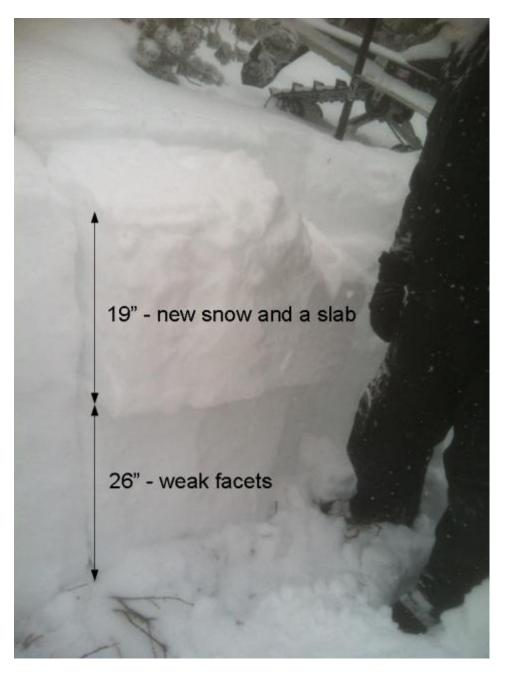
This snowpit in the Cabin Creek area of the Southern Madison Range has a total snowpack depth of almost 4 feet. The bottom 2 feet is all weak, sugary facets and the upper 2 feet is a slab. See the complete snow profile graph <u>here</u>. Photo: B. Radecky
