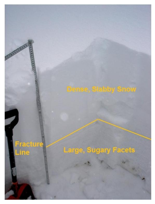
A natural avalanche released on the layer of big, faceted grains. The slab was up to 2 feet thick. This snowpack stricture is similar throughout southwest Montana. Slab + Weak Layer + Steep Slope + Trigger = Avalanche.
