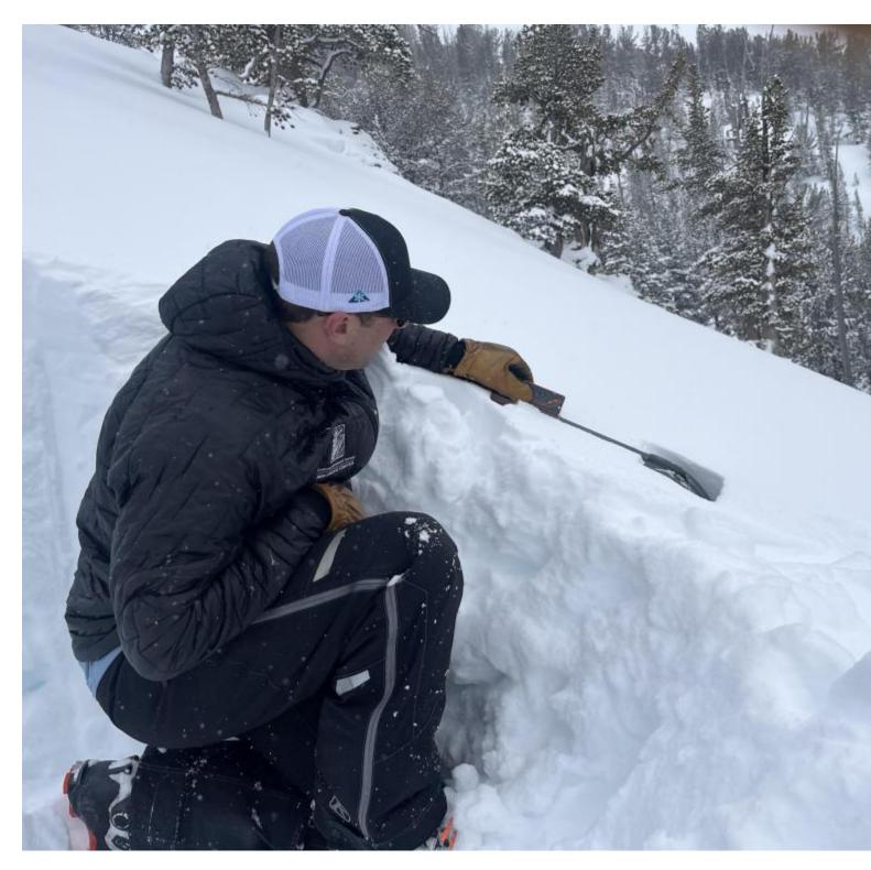
Checking the slope angle on the west side of Henderson Mountain outside Cooke City. Selecting terrain less than 30 degrees steep is the most reliable way to avoid avalanches. The most reliable way to know the slope angle, measure it. Photo: GNFAC
