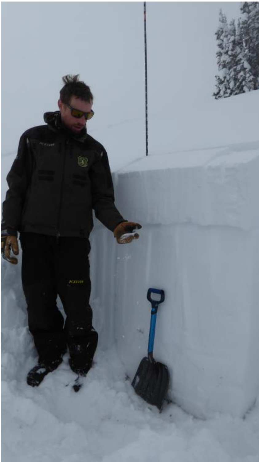
Alex Marienthal points a 5 cm thick weak layer of faceted snow that broke with an ECTP10. Photo: GNFAC
