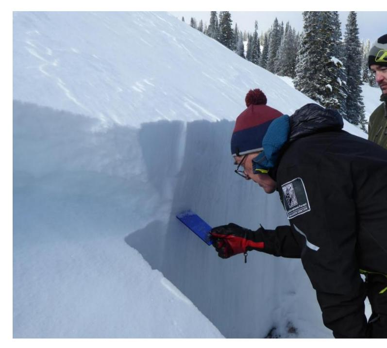
Identifying snow crystals in the layer that failed at the crown of the avalanche on Ski Hill. The avalanche broke on weak, faceted crystals near the surface. Photo: GNFAC
