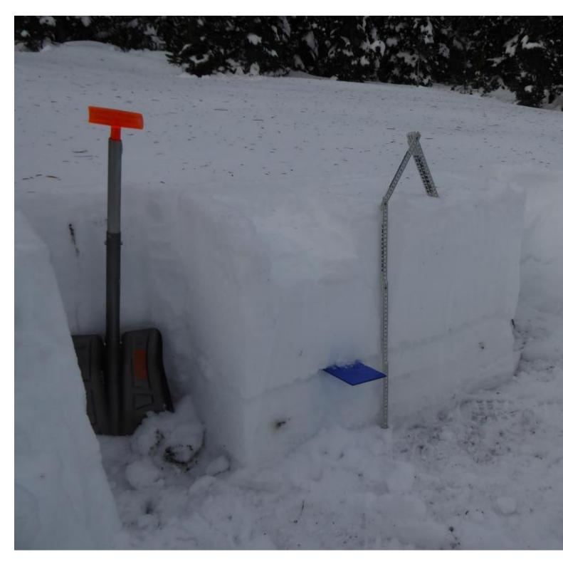
The snow was breaking 1 foot off the ground in the layer at the blue crystal card. Weak, sugary snow broke and propagated in the extended column test with 18 and 21 taps. We anticipate this weakness to get worse in the coming weeks. Photo: GNFAC
