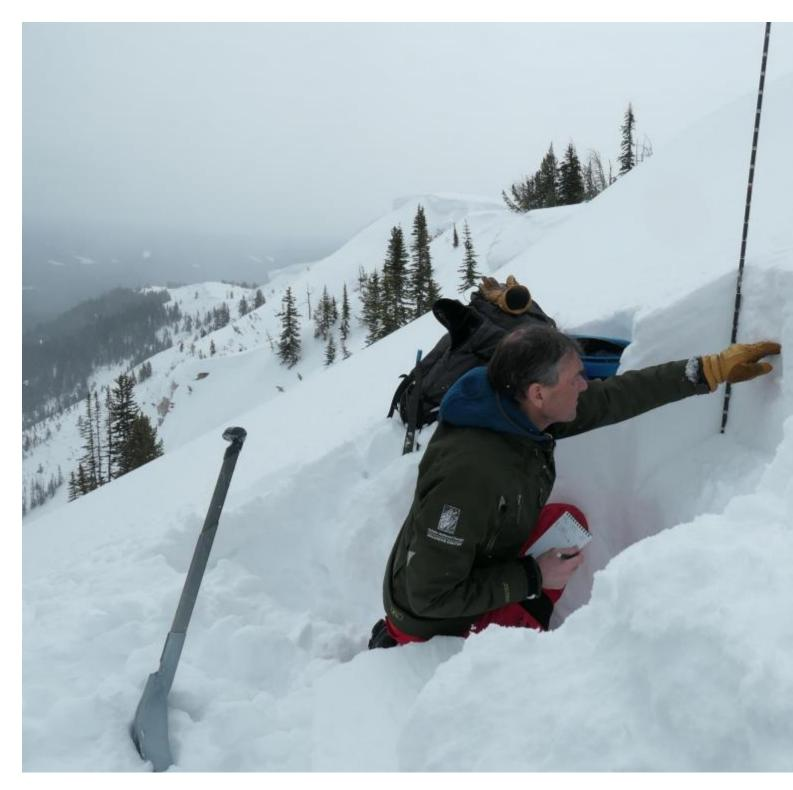
Today on the east side of Lionhead Ridge we found a layer of weak, near-surface facets buried under a foot and a half of new snow. This is definitely something to watch out for especially on wind-loaded slopes. Photos: GNFAC
