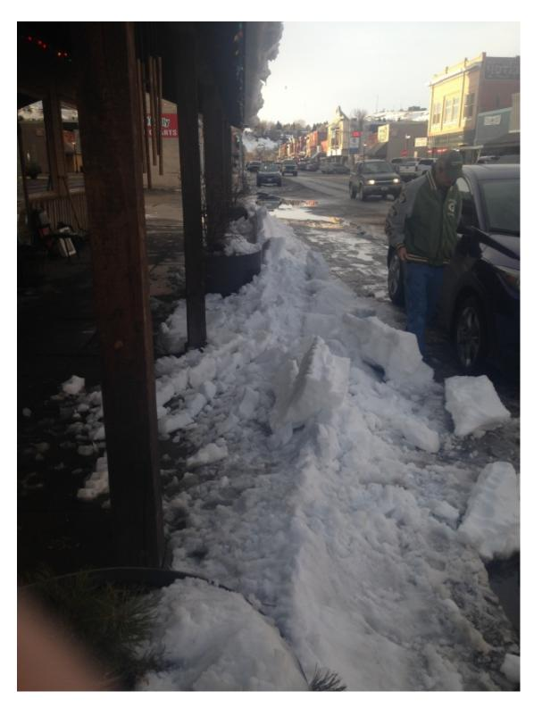
Low angle metal roofs have heavy, thick slabs of snow that built up during persistent cold temperatures. These slabs will slide during warm temperatures. Be on the lookout for overhead hazard and be cautious where you walk or park your car during warm sunny days. An additional urban hazard are large icicles are that will break during warm days. Photo: A. Schauer
