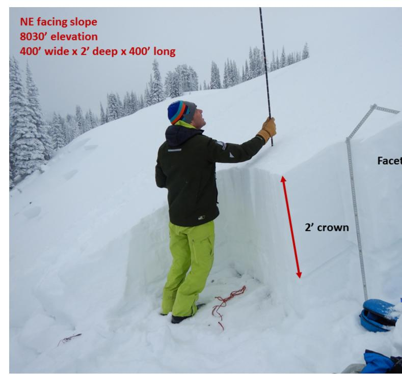
The avalanche failed on a thick (10cm) layer of facets that were sitting on an ice crust. The slide was a natural soft slab avalanche that broke with just a few new inches of snow and wind. Photo: D. Zinn
