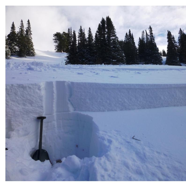
This avalanche broke on small facets that formed at the snow surface before the recent snows. This small hill is very steep (>45 degrees) and wind-loaded. It was triggered by a dog. The main trail is about 50 feet uphill of the crown. Photo: GNFAC
