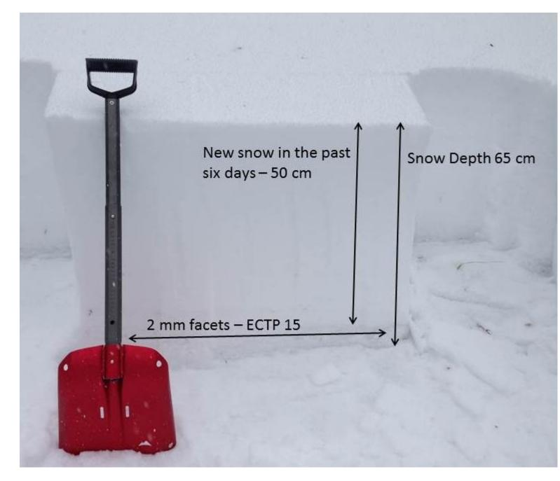
This pit was dug on a NE facing slope at 8,000 ft. north of Bridger Bowl. Facets near the ground continue to propagate in stability tests indicating an unstable structure. Photo GNFAC
