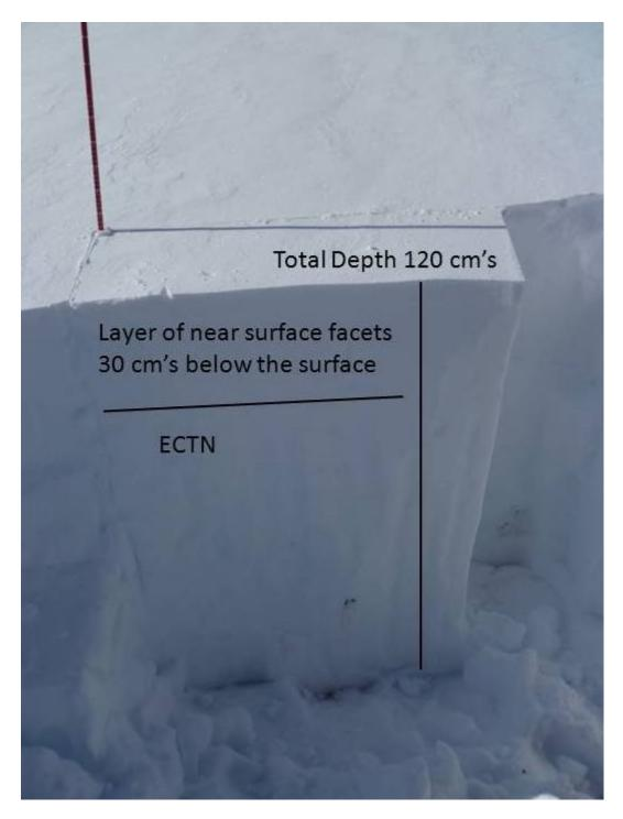
A layer of near surface facets that formed in early January did not produce unstable results in stability tests. This pit was dug on a NE facing slope around 9000 ft. This layer exists in many locations throughout the southern portions of our forecast area. Although it appears to be gaining strength, this layer should be looked for and assessed before committing to steep slopes. Photo GNFAC
