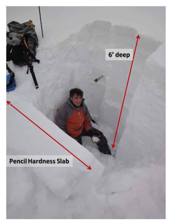
This pit was dug on a northwest facing slope at 8,750' in Lionhead. A dense, six foot thick pencil hardness slab is being supported by fist hardness depth hoar. I scooped out some in my hand. The column broke on this layer and I was able to lay the pillar, intact, outside the snowpit. The deeper the depth hoar gets buried, the more difficult it becomes to trigger. But if you get unlucky and trigger it the avalanche will be large, destructive and deadly. Photo: GNFAC
